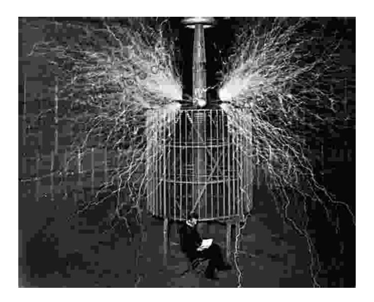
The Tesla coil is a high-voltage transformer that produces alternating currents of very high voltage and low amperage. Tesla developed the Tesla coil in the late 1890s as a means of generating artificial lightning. Today, Tesla coils are used in a variety of applications, including medical imaging, particle accelerators, and plasma research.
